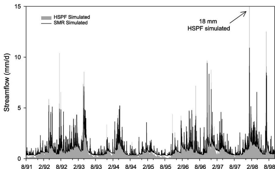
Fig. 6. HSPF and SMR simulated streamflow of Irondequoit Creek at Railroad Mills during the seven-year simulation period.
