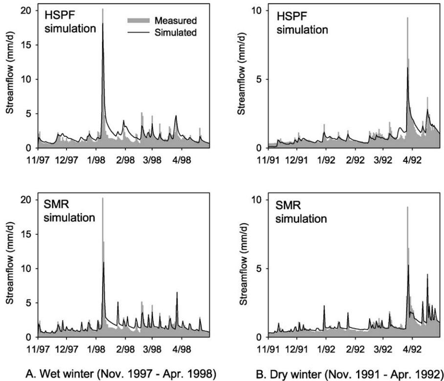
Fig. 7. Measured and simulated (HSPF and SMR) streamflow of Irondequoit Creek at Railroad Mills during representative wet and dry winters. A. Wet winter (November 1997–April 1998). B. Dry winter (November 1991–April 1992).
