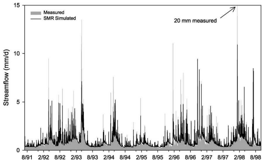
Fig. 5. Measured and SMR simulated streamflow of Irondequoit Creek at Railroad Mills during the seven-year simulation period.
