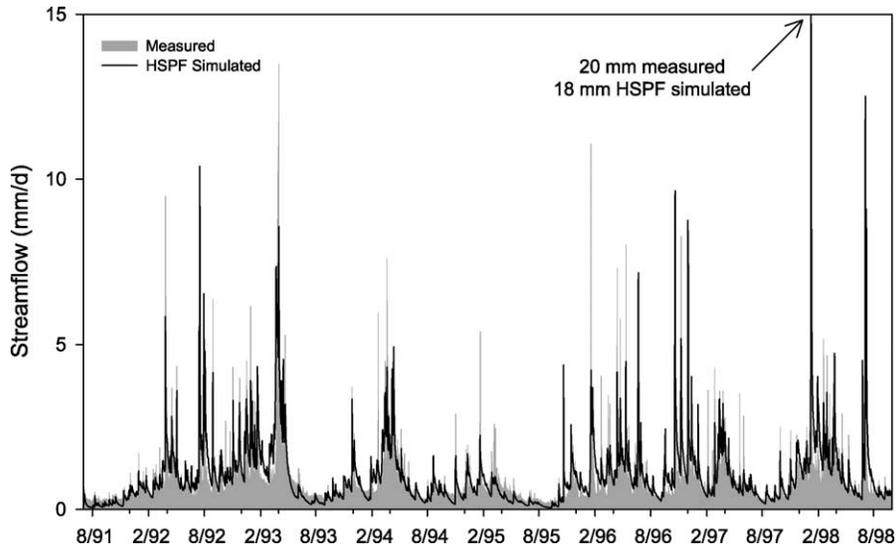
Fig. 4. Measured and HSPF simulated streamflow of Irondequoit Creek at Railroad Mills during the seven-year simulation period.
