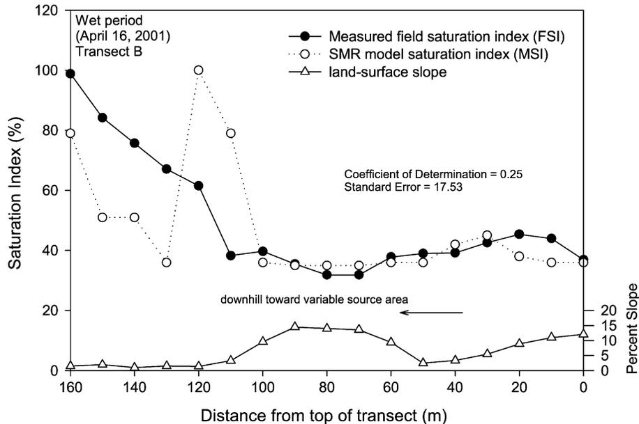
Fig. 10. Field and SMR simulated soil-saturation indices in the Irondequoit Creek basin: Representative wet period (April 2001) along transect B.
