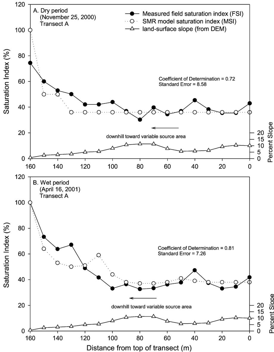
Fig. 9. Field and SMR simulated soil-saturation indices in the Irondequoit Creek basin. A. Representative dry period (November 2000) along transect A. B. Representative wet period (April 2001) along transect A.
